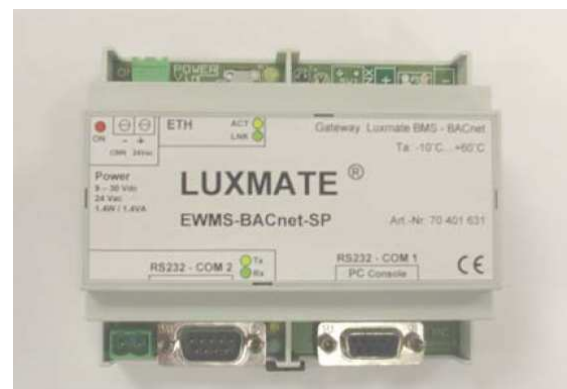
Pasarela BACnet IP.
