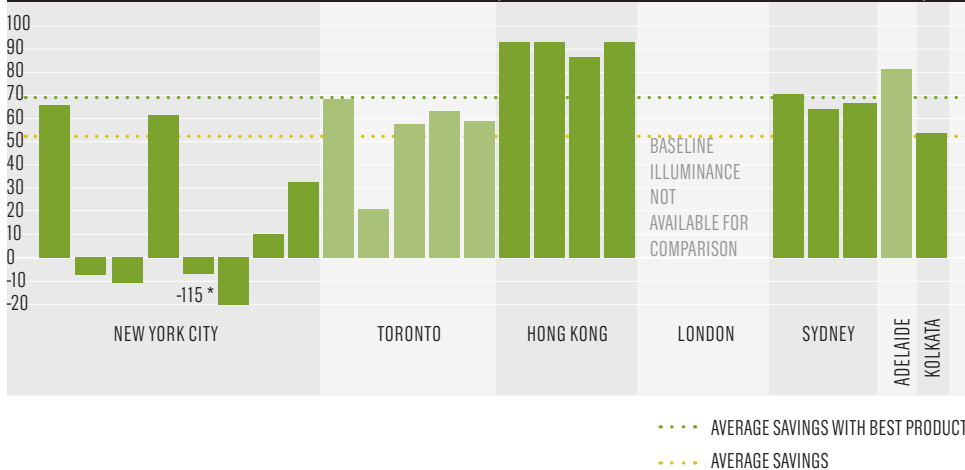
FIGURE 6 PERCENTAGE ENERGY SAVINGS PER UNIT LUX PRODUCED (NORMALIZED, BASED ON FIRST 3000-6000 HOURS OF DATA)
